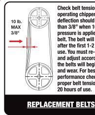
Check belt tension before operating chipper. Belt deflection should be less than 3/8" when 10 lbs. of pressure is applied to the belt. The belt will relax after the first 1-2 hours of use. You must re-check and adjust accordingly or the belts will begin to slip and wear. For best performance check for proper belt tension every
